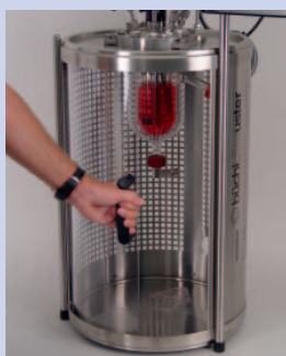
Polycarbonate protection door for optimal user safety
