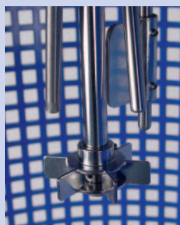
Turbine stirrer with gasing stirrer shaft for effective gas dispersion
